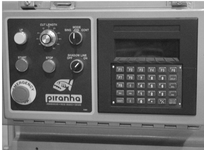
Figure 3: Main Control Panel-Programmable CNC
