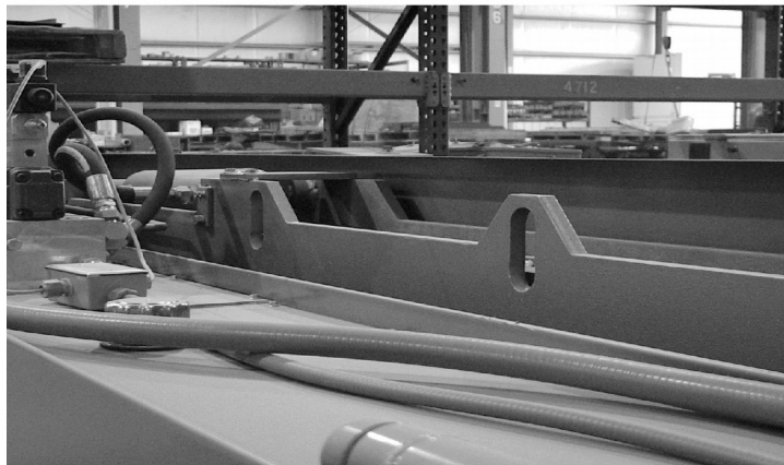
Figure 1: Lifting Lug Location
