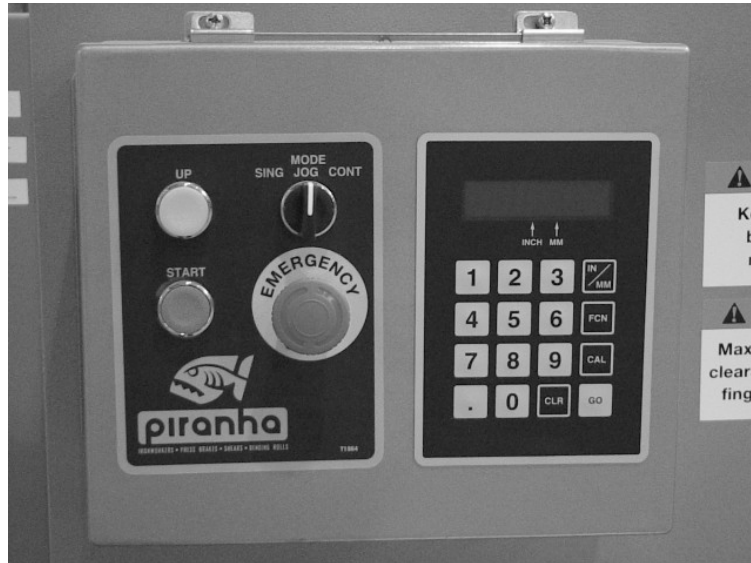
Figure 4: Main Control Panel-Programmable GOTO
