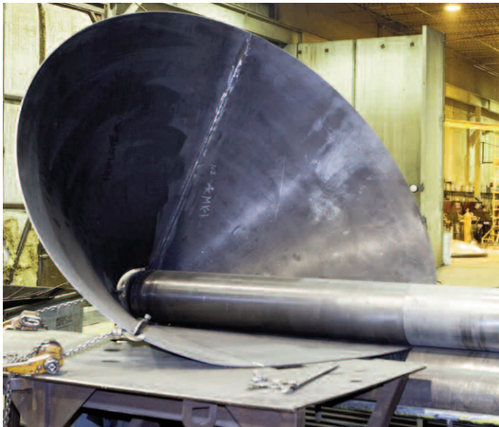
Wilco's Bertsch Plate Roll forms a cone from 5/8" steel going from a 96" down to an 18" diameter
