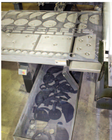
Type, size and configuration of parts from a plate very greatly. Production continues while most parts are automatically removed via the 3400 XP drop door and parts conveyor.
