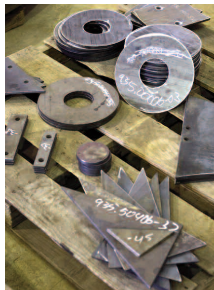
Type, size and configuration of parts from a plate very greatly. Production continues while most parts are automatically removed via the 3400 XP drop door and parts conveyor.
