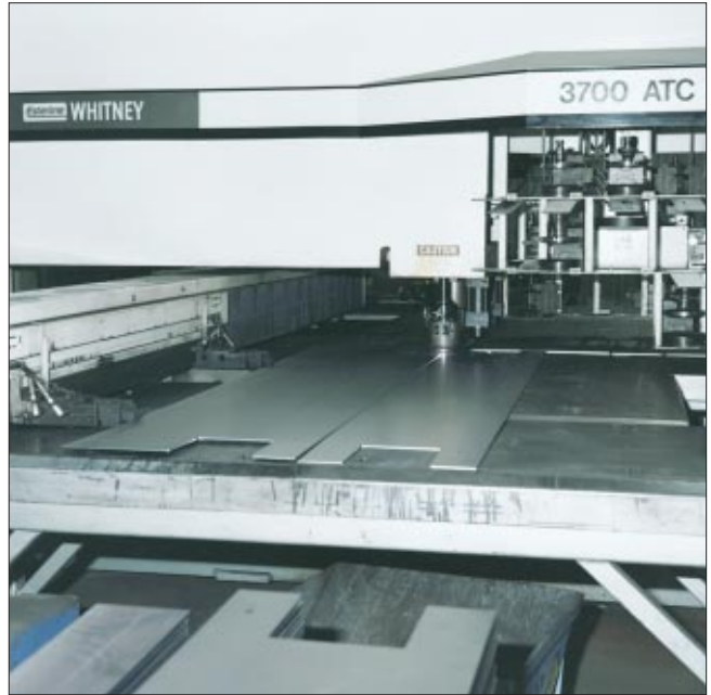
Dross-free cuts on the W.A. Whitney 3700 ATC produce quality parts without secondary operations.
