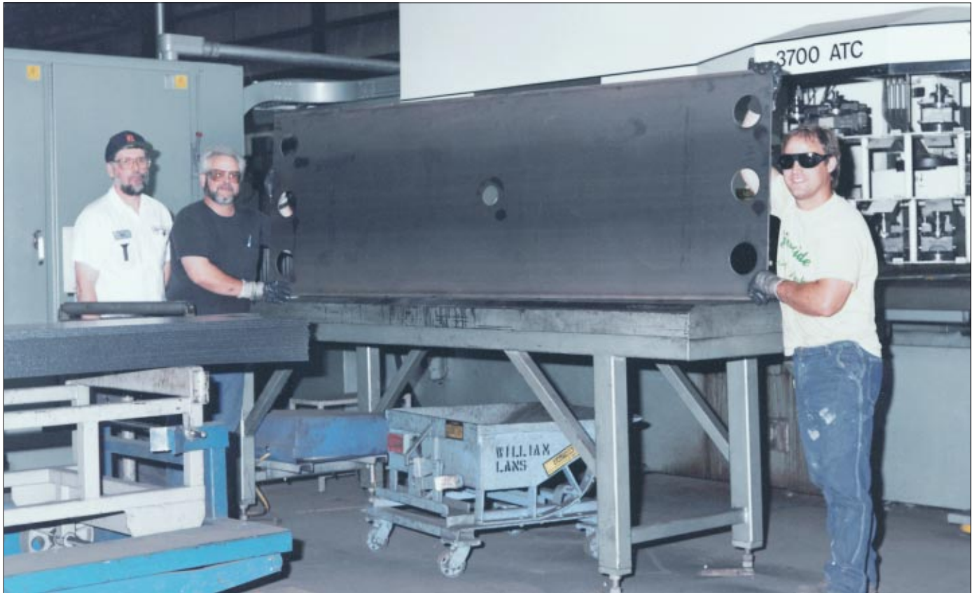
Tim Reilly, Ron Hinds and Don Hasselberger displaying a Tower King Pin Plate fabricated on the 3700 ATC. Stoughton produces many large parts off the 3700 ATCs.
