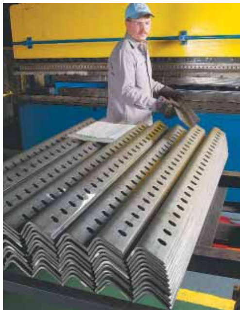
Jason Cook bends the fifth wheel angles into their final form.
