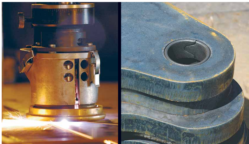
Left: Plasma cutting with 400 amps. Right: Compression bushings are pressed into a punched and shaved hole at the 4400 MAX.
